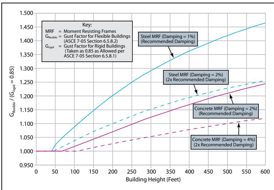
Figure 3: Effect of Building Flexibility on Gust Factor for 100-foot x 100-foot Building.
