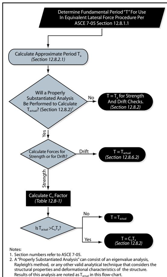
Figure 1: Seismic Equivalent Lateral Force Fundamental Period Flow-Chart.
