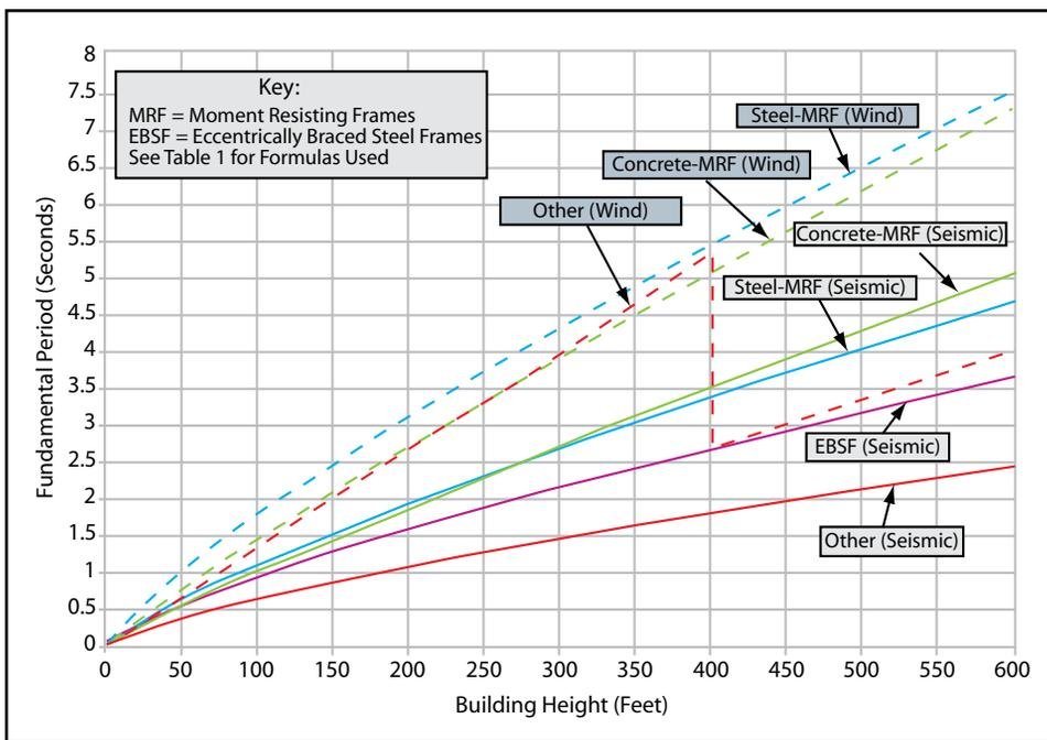
Figure 2: Approximate Fundamental Period vs. Building Height.
